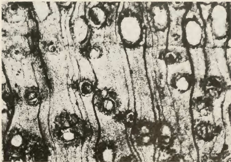
Fig. 4: Cross section. Growth ring boundary with marked differences in vessel diameter between late wood and early wood of the following ring. \times 50 .
